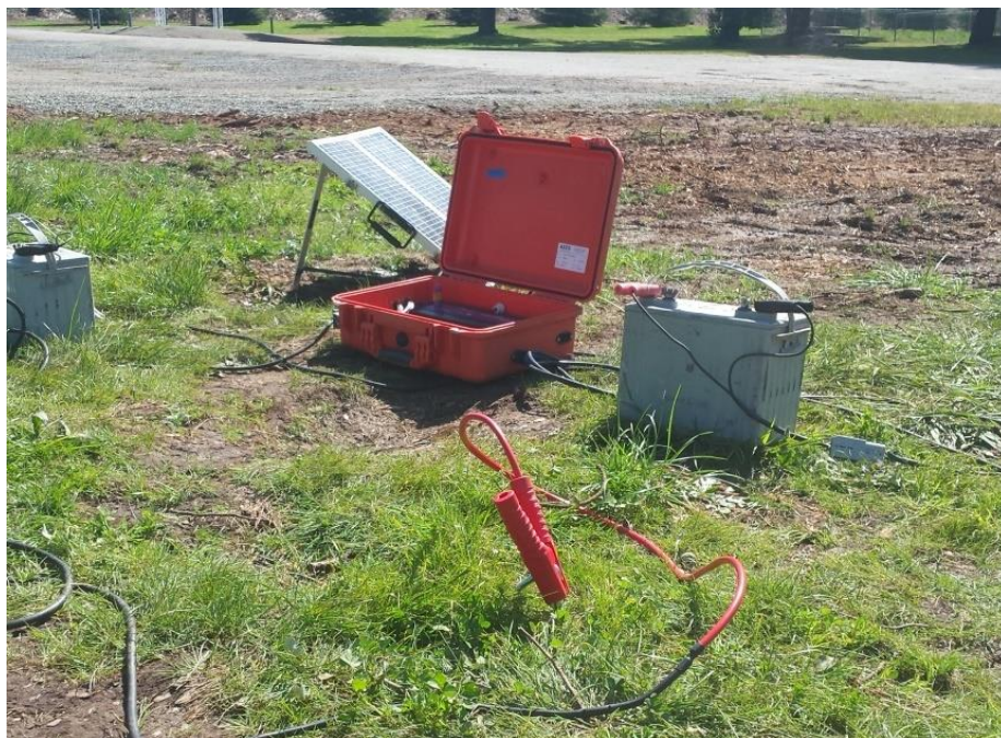
Figure 3: SP field logger set up used for the survey. The SP data taker box (centre) is connected to both a battery power source as well as solar panels (either side) to ensure power is supplied throughout the test. Modified seismic cables are utilised (black cable); with the modified jumper lead connectors seen in the foreground being attached to the metal stakes acting as electrodes in the ground. An individual SP field logger was utilised for each line.
