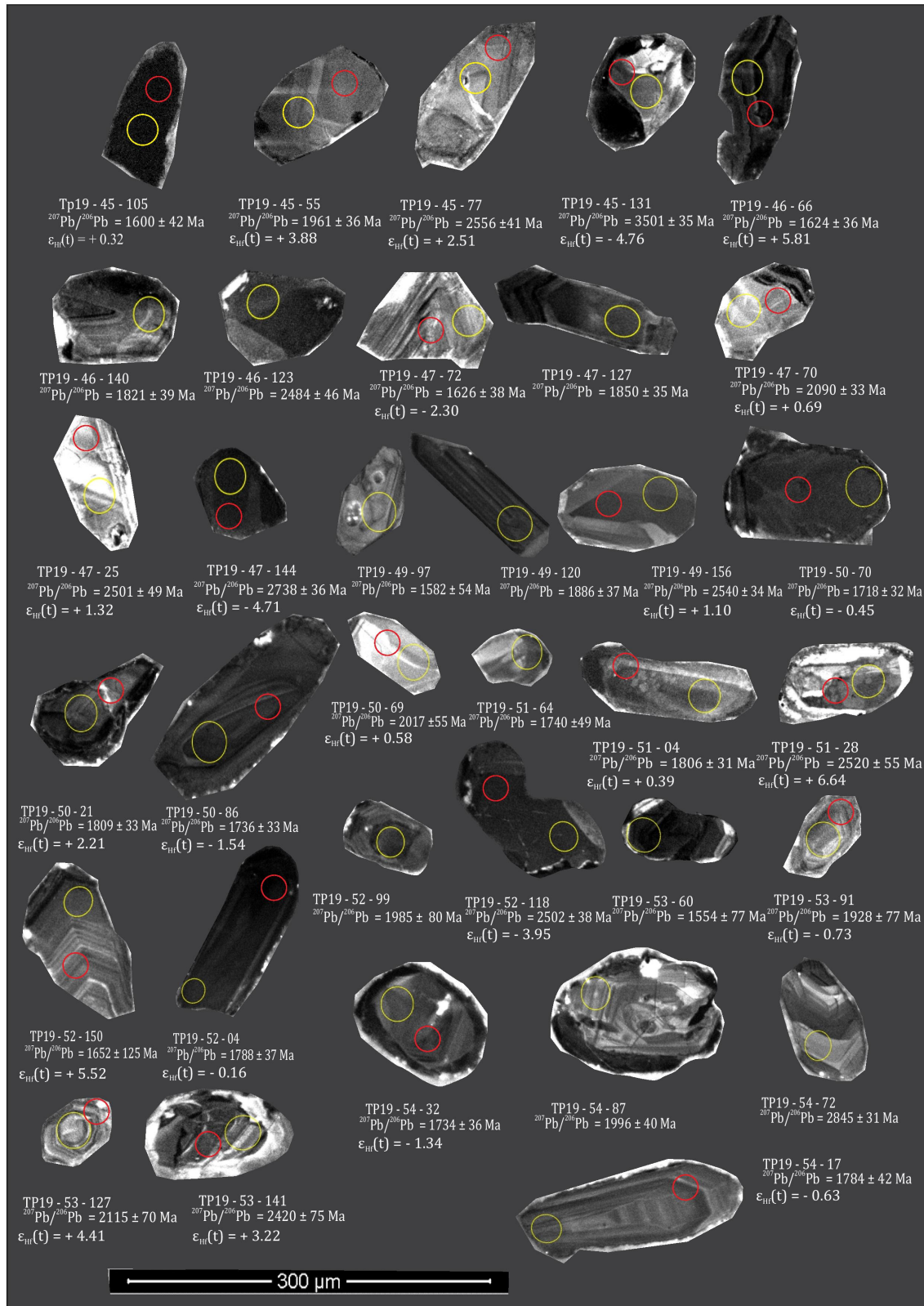
Figure 5. Cathodoluminescence (CL) images of zircons from the Renner Group with their associated ^{207}\text{Pb}/^{206}\text{Pb} age. The red circles show the location of U-Pb spots and the yellow represents the Lu-Hf spots.
